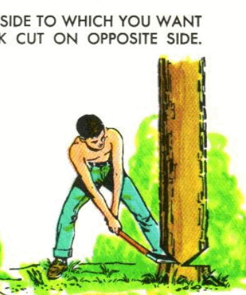
6. MAKE DIAGONAL CUT FIRST. THEN HORIZONTAL BOX CUT. NEXT CUT THE OTHER SIDE.
